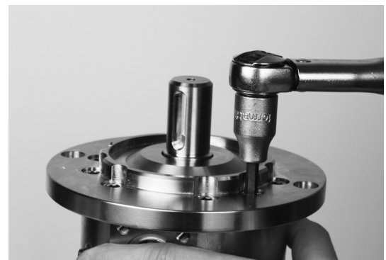
40. Tighten with 30 Nm
