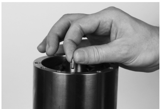
24. Mount 1 guide pin in pump housing
