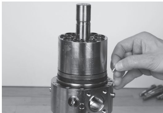
21. Raise pump to vertical position and remove 1 guide pin
