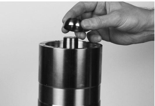
19. Mount retainer ball on top of the spring
