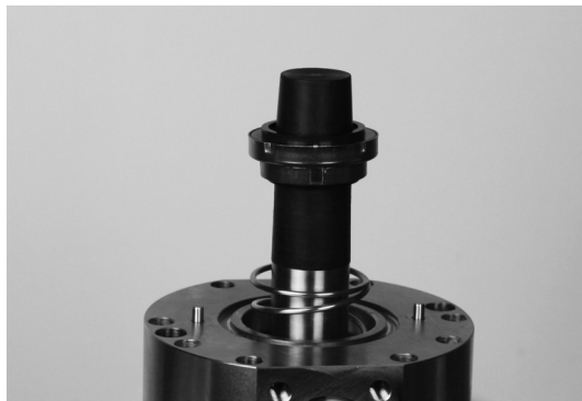
36. Mount shaft seal in flange
