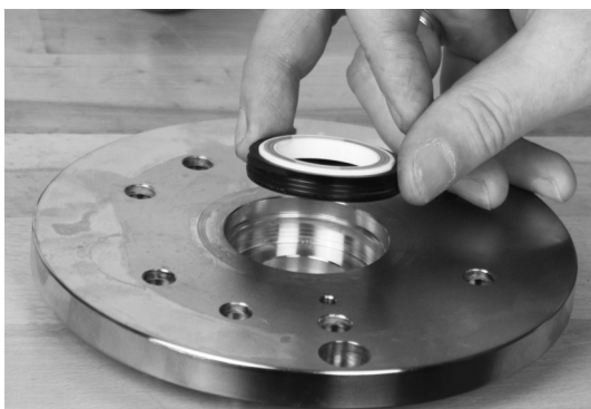
36. Mount shaft seal in flange
